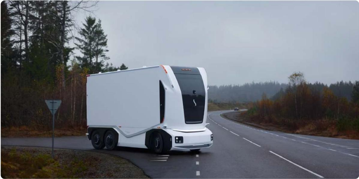
**i** Autonomous Gen 2 - Einride's latest electric powered and autonomous shipping truck (Photo: Einride)
